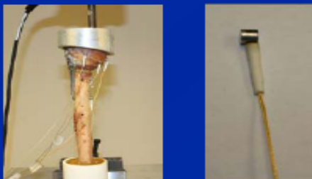
Fig. 1 Mechanical testing setup (left) and AE sensors (right).
