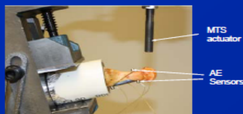
Figure 1: Experimental setup with four AE sensors attached on the specimen surface.
